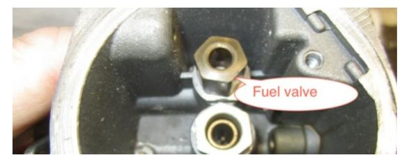
Then you need to pull out the fuel inlet pipe that is fitted. You will be reusing this so do not damage it. It is only a press fit into the casting, so use a 5mm tap to grip the inside of the tube firmly and then pull out.
