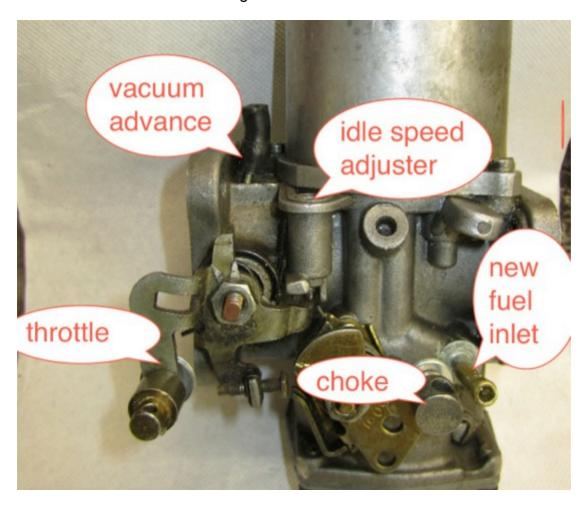
Remove the dashpot cover and piston. Install the correct BBA needle and set the carb
