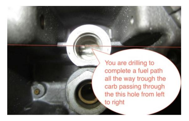
Press the carefully extracted fuel inlet tube into the new hole and then plug the vacant hole with a piece of brass dowel. Both these pressings must be tight to avoid fuel leaks.
