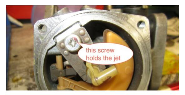
Then remove the float by unscrewing the screw on the body of the carb
