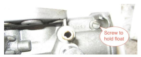
Now remove the needle valve with a  $\frac{1}{2}$  inch socket – the needle is already loose so do not lose it
