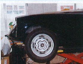
8 Shell finally meets chassis for painting.
