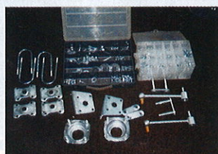
6 Numerous metal bits are blasted and nickel-plated.
