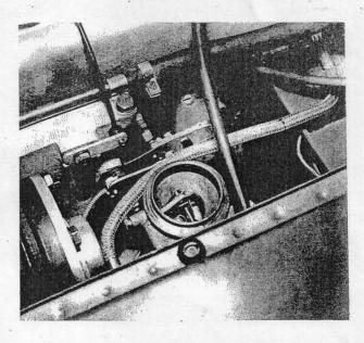
8. Push gas line into position as shown in illustration and tighten 1/2" fuel line bolt on side of carburetor.
